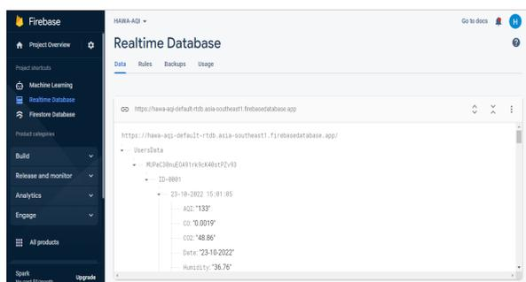
Figure-11. Real-time nodes in Google Firebase
