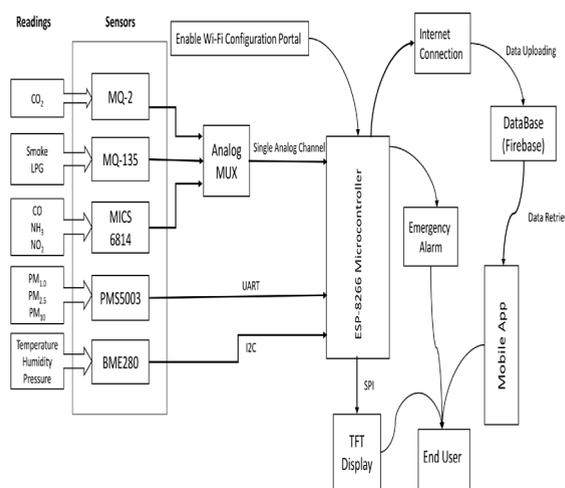
Figure-3. System Block Diagram
